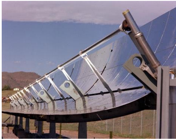
Figure 6: Thermodynamic unit with linear parabolic mirrors
